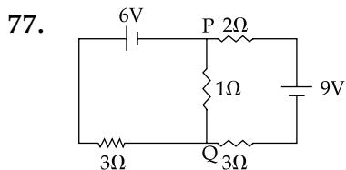
In the circuit shown, the current in the  $1\Omega$  resistor is :
