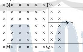
A rectangular loop PQMN with movable arm PQ of length 15 cm and resistance 4  $\Omega$  is placed in a uniform magnetic field of 0.25 T acting perpendicular to the plane of the loop as is shown in the figure. The resistances of the arms MN, NP and MQ are negligible. Calculate the (i) emf induced in the arm PQ and (ii) current induced in the loop when arm PQ is moved with velocity 25 m/s.
