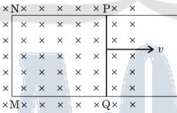
A rectangular loop PQMN with movable arm PQ of length 10 cm and resistance 2  $\Omega$  is placed in a uniform magnetic field of 0.1 T acting perpendicular to the plane of the loop as is shown in the figure. The resistances of the arms MN, NP and MQ are negligible. Calculate the (i) emf induced in the arm PQ and (ii) current induced in the loop when arm PQ is moved with velocity 20 m/s.
