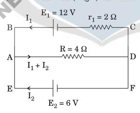
In the electric network shown in the figure, use Kirchhoff's rules to calculate the power consumed by the resistance  $R = 4 \Omega$ .
